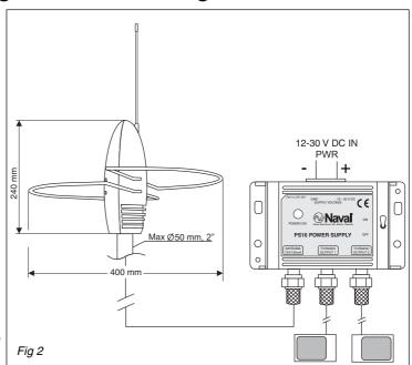
Install the fuseholder with a T400 mA fuse in the positive branch of the power cable. If AC is required please use a local adapter.
