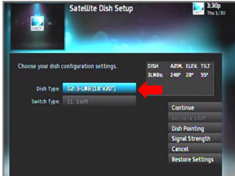
Figure 5-4 Satellite Dish Setup on DIRECTV Receiver
