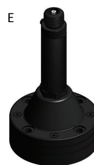
E NATO 4-hole Rigid (no spring) 4 x M10 or 3/8" Bolts on 114mm PCD Base diameter 140mm
